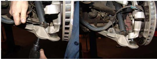
Figure 5 Separation of the front lower control arm
