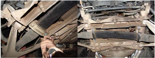
Start by removing the driver side first as this has the control arm removed and will take the remainder of the pressure off of the spring. Move to the passenger side and pull the spring from the car.
