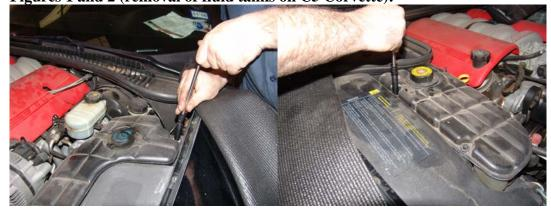
Once the tanks have been moved from their mounts, you can now access the shock top mounts on the factory shocks. This can be done with a special Snap-On socket, or you can loosen the nut with a ratchet, if the shock piston starts to turn you will have to hold the shock with a wrench, while loosening the nut with another.
