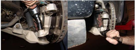
You will only be removing one lower control arm and upright, one on the front and one on the rear. You may now also remove the shock from the passenger side of the car. Make sure that all rubber shock mounts have been removed from the chassis side of the car as well at this time, these will not be needed.
