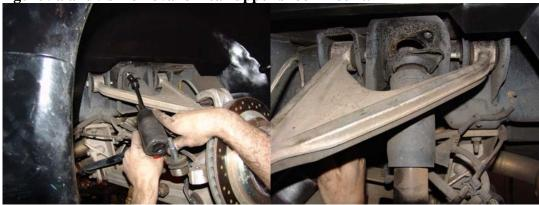
Pull the shock free, and clean off any debris that might be on the frame. We have now completely removed the shock and spring system from the car and are ready to install our new LG coil over suspension package.
