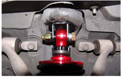
Once the upper portion of the shock is mounted we can now lift the lower control arm up to insert the supplied bolts. Make sure that the upper mount is facing how you see in figure 10. This way the shock can pivot through the suspension travel correctly and you can easily see the adjuster.
