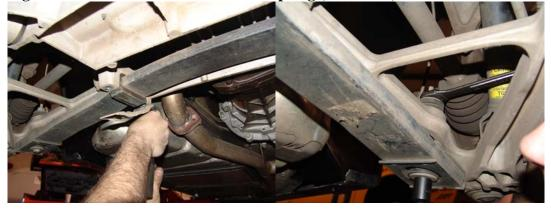
Now that the spring has been removed, take the upper shock mounts loose from the car and remove the rear shocks. This is done by removing the two 10mm bolts holding the upper shock mount plate to the frame of the car.
