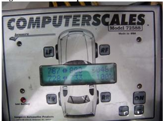
Keep in mind, you can not change front, rear, or side percentage without physically moving, adding, or removing weight. The cross can be adjusted by changing the spring adjusters on the shocks. This change will make sure the car handles the same at the limit on both right and left hand corners.
