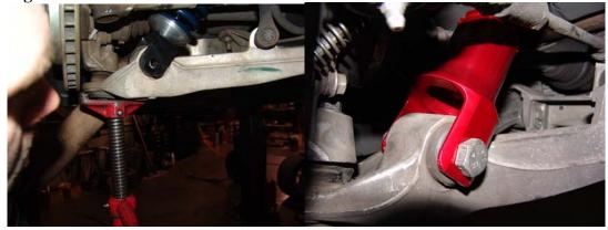
Finish the install by installing sway bar end links, and making sure all mounts, nuts, bolts, are tight. Also make sure that all wires, and fluid lines are clear of the springs and shocks so that they are not pinched.
